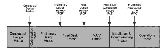
Figure 3. 4MOST Project phases and main reviews. Note that the *Operations Phase* is beyond the scope of the 4MOST systems engineering and it is shown for the sake of completeness
