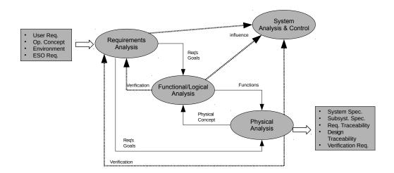
Figure 2. 4MOST System Engineering design approach<sup>2</sup>
