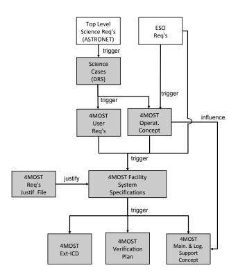
Figure 6. 4MOST Top Level Requirement Documentation. Documents external to 4MOST are showed in white
