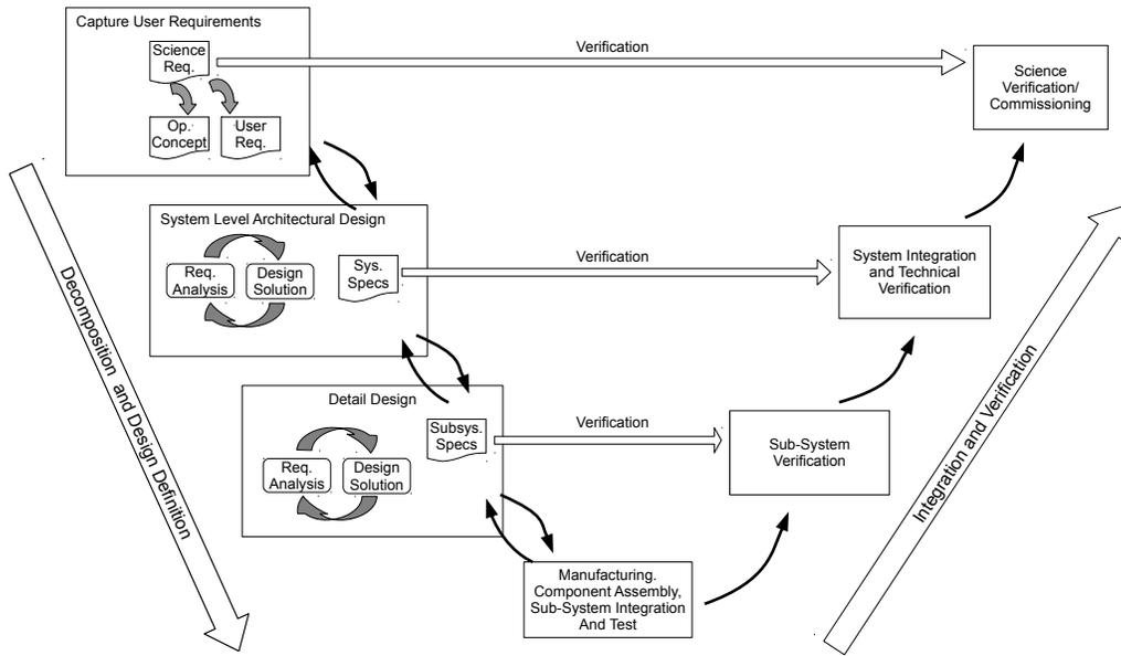
Figure 1. 4MOST System Engineering Process Vee Model
