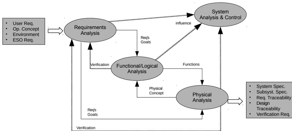
Figure 2. 4MOST System Engineering design approach<sup>2</sup>
